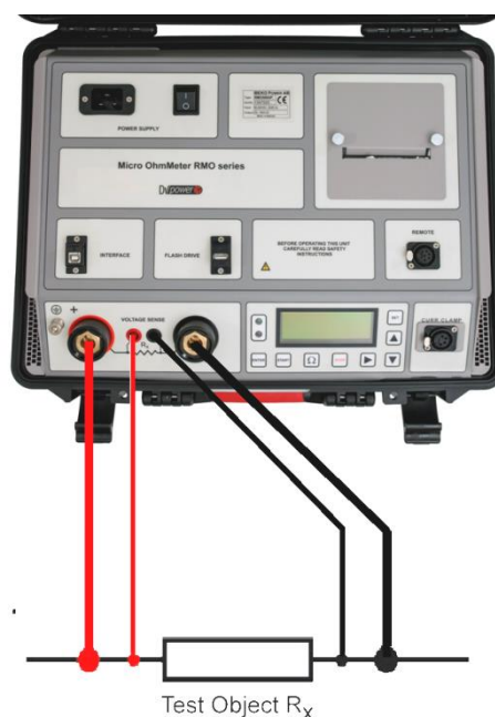
Figure 3-1: Connecting test object to RMO-G
