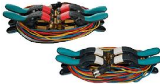
Figure 3-12: H cables’ TTA clamps with red tape attached (upper) and X cables’ TTA clamps with white tape attached (lower)
