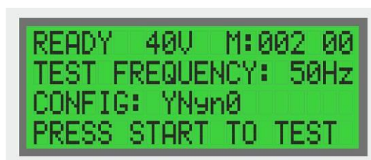
Figure 4-5: The READY screen before the test
