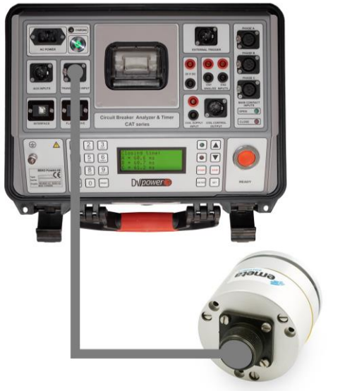
Figure 3-11: Connecting a rotary digital transducer to the CAT
