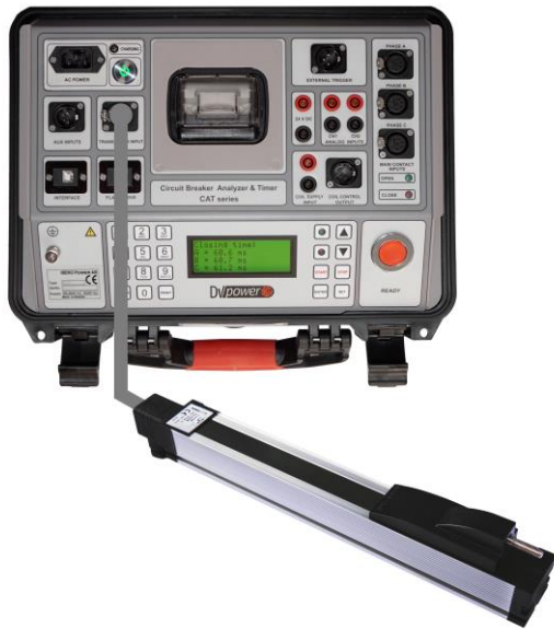
Figure 3-9: Connecting a linear analog transducer to the CAT
