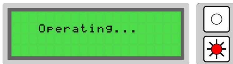
Figure 3-28: Operating message and LED indication
